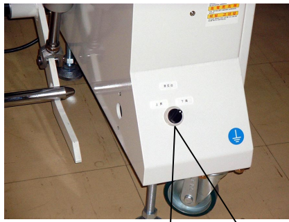
Fabric lifter activates with this switch turned ON after rolling-in the fabric onto the lifter arm.
